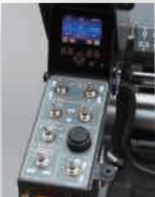
Screed control box
