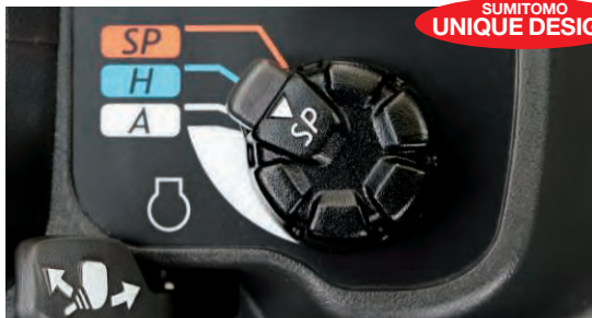
Integrated Throttle Mode Selector The throttle mode can be selected by simply turning the knob, so anyone can easily choose the optimum working mode.
