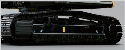
Full Track Guard A full track guard along the lower undercarriage prevents shoes riding off, and also helps to protect the rollers.
