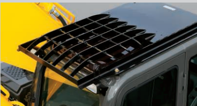
Front Guard & Head Guard (OPTION) A front guard and head guard is available to protect the cab from falling rocks or debris.
