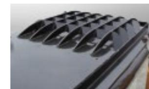
FOPS-Falling Object Protective Structures
