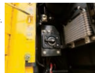
Central fuse box located behind seat Easy-access AC filter Washable cab floor and floor mats
