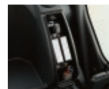
Central fuse box located behind seat
