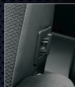
Seat heater switch
