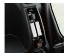
Central fuse box located behind seat
