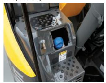
Urea Tank Capacity: 43 L Refilling frequency: Once per 7 refuellings
