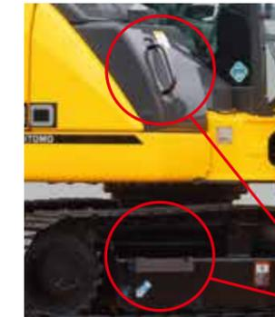
ISO compliant hand grip and lower step allow easy access to the upper structure. Shape of the right-hand corner cover has been optimised for better visibility from the cabin.
