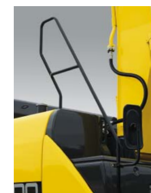
ISO-compliant large handrail
