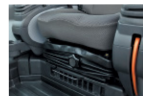
The Suspension Seat Eliminates Vibration.
